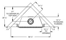
These dimensions allow for 1" of clearance at the sides and back of fireplace. 0" clearance is also permitted at all sides if framed.
